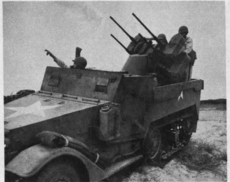
Angular hood of M-3 half-track chassis can be seen in this close-up view of an M-16. The rear drive has a single bogie carrying four small wheels, a large forward driving sprocket and idler at the rear.
